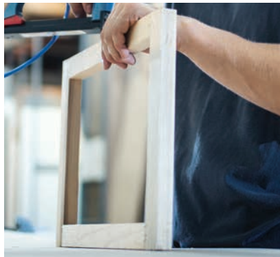
Butt-joint glued and stapled
